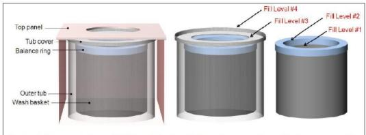
Figure 1: Representation of Fill Levels for the Clothes Container Capacity Measurement for Vertical-Axis Clothes Washers
